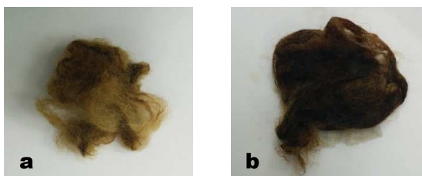
Fig.3a: Untreated Merino wool fiber, 3b: Plasma treated Merino wool fiber
