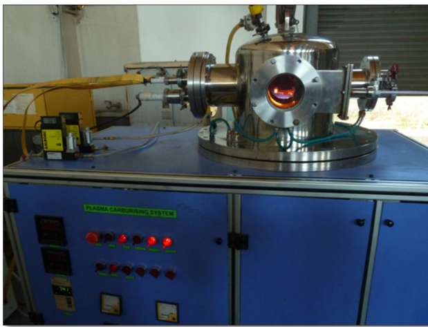
Fig. 1: Plasma carburizing system installed at FCIPT
