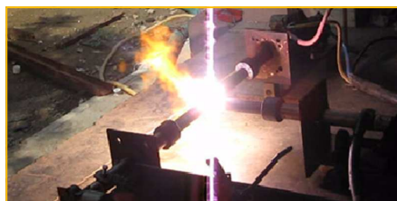
Graphite plasma arc system generates high temperature
