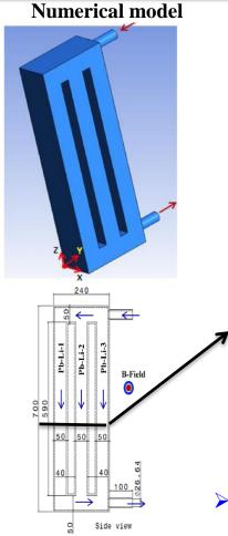
2D view of model along with dimensions (in mm)
