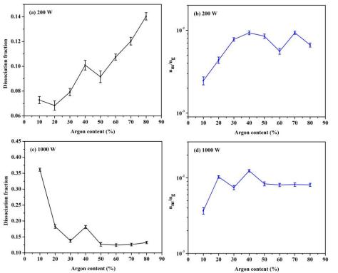
Fig: Variation of dissociation fraction of nitrogen molecule for (a) 200 W and (c) 1000 W and argon metastable fraction for (b) 200 W and (d) 1000 W of applied RF power against the argon concentration at  $5 \times 10^{-3}$  mbar working pressure.
