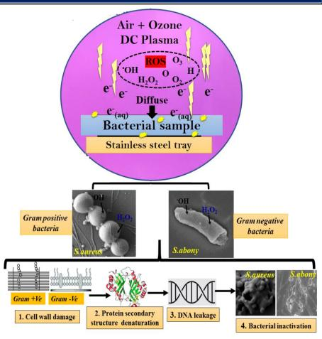
Figure: Schematic demonstration of bacterial inactivation by plasma
