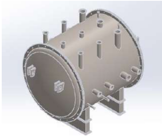
Fig 6: Isometric view of conceptual design without support assembly
